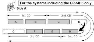
The tune interrupted in the middle at the end of tape side A is erased and side B starts from the beginning of that tune. (Up to 32)
